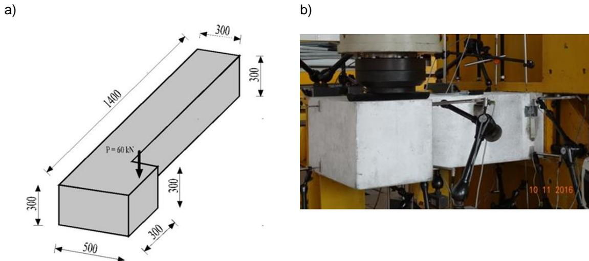
Fig. 1 Analysed cantilever beam, a) geometry and reinforcement of tested beams, b) the view of the test stand
