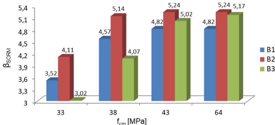
Fig. 2 The impact of concrete strength on the reliability index of complex beam reliability systems
